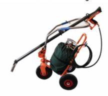
The high velocity heat generated by the thermal extension lance evaporates moisture in weeds by "thermally shocking" them. This causes weeds to die naturally by exploding their cells. A propane tank (not included) is required.
