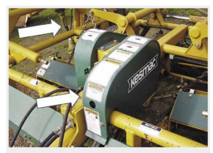
Here, you can see the chains and sprockets are properly guarded, yet the spinner shaft shield on the mower head is broken and is no longer protecting workers from entanglement. Photo by Jary Winstead.
