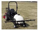
Hasty Vac The zero-turn Z200 has a 35-gallon poly tank, no-drip TeeJet tips, 12-volt pump, 10-inch pneumatic casters, inline strainer and three-section breakaway boom.
